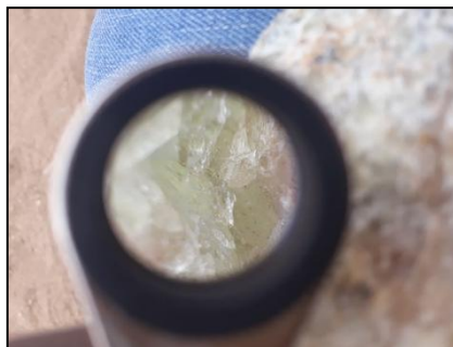
Figure 6-13: Massive to prismatic crystals of translucent yellowish apatite with a vitreous to silky luster (sample from Mariela mine drillings with 20x magnifying glass).
