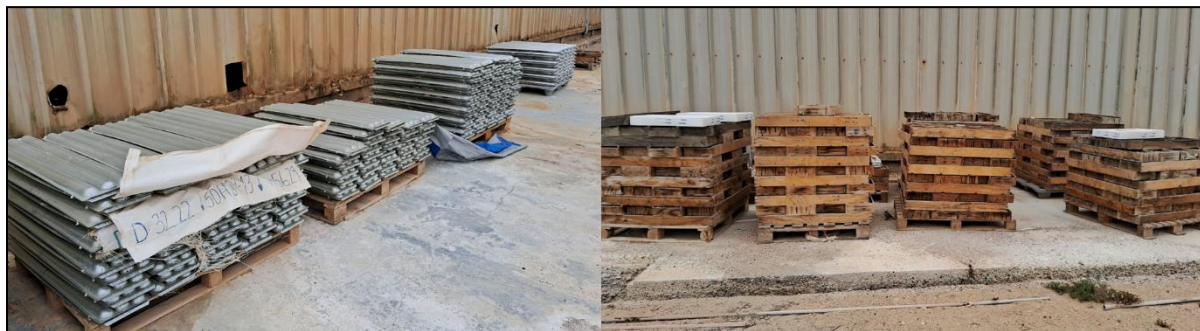
Figure 6-18: Final arrangement of the drilling boxes. Left: cut sections transferred to metal boxes. Right: uncut sections kept in the original box.
